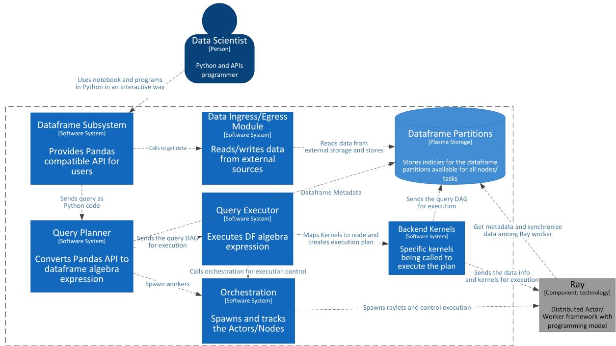
For the simplicity the other execution systems - Dask and MPI are omitted and only Ray execution is shown.
