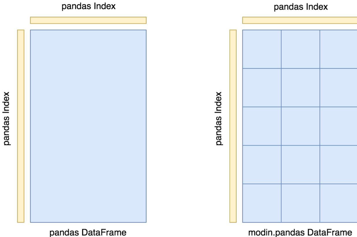
Currently, the main in-memory format of each partition is a [pandas DataFrame](#) (pandas storage format). HDK, PyArrow and cuDF are also supported as experimental in-memory formats in Modin.
