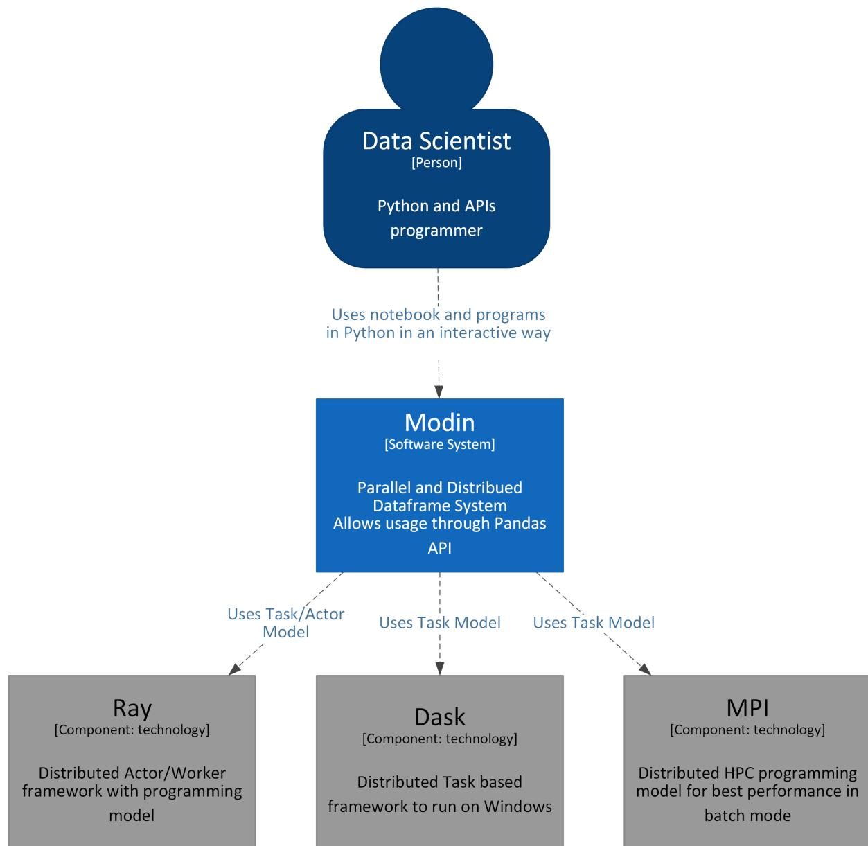
The user - Data Scientist interacts with the Modin system by sending interactive or batch commands through API and Modin executes them using various execution engines: Ray, Dask and MPI are currently supported.
